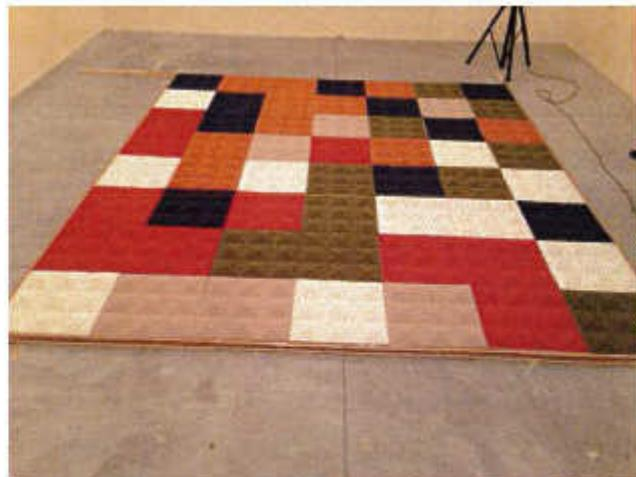
**Test specimen description:** panel mod. "STILLY" (nominal size 440 mm x 440 mm, maximum height 40 mm, mass 0,4 kg) composed of a plastic support frame and polyester felt (6 mm thick) lined with Trevira polyester tissue.
